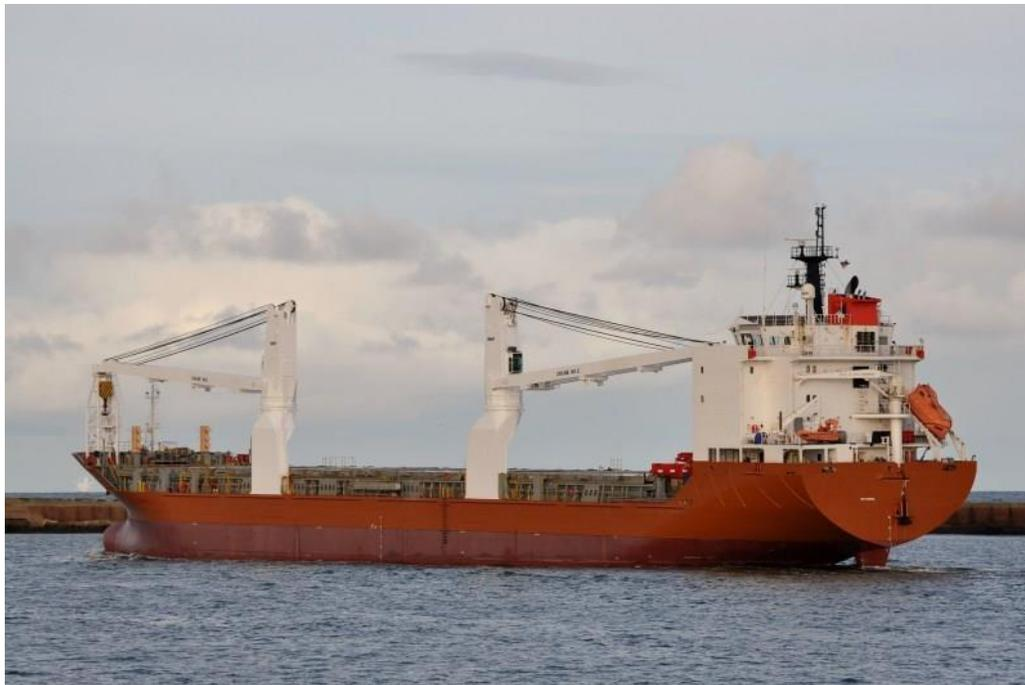
The MV Nunalik is the latest addition to the growing NEAS fleet of modern vessels serving Canada's Arctic communities. At 138 meters length, the new vessel is an ice class 1, multi-purpose, tweendecker that offers specialized cargo and advanced heavy-lift handling technologies.
