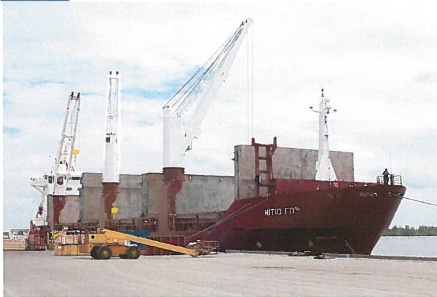
The MV Mitiq is the latest addition to NEAS' growing fleet of modern vessels serving Canada's Arctic communities. At 137 meters length, the new vessel is an ice class 1, multi-purpose, tweendecker that offers specialized cargo and advanced handling technologies.
