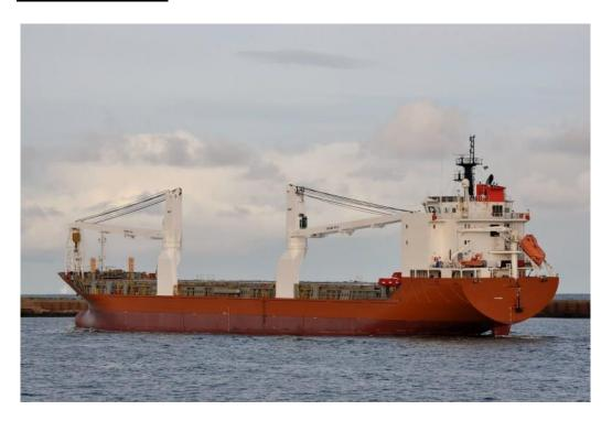
The MV Nunalik is the latest addition to the growing NEAS fleet of modern vessels serving Canada's Arctic communities. At 138 meters length, the new vessel is an ice class 1, multi-purpose, tweendecker that offers specialized cargo and advanced heavy-lift handling technologies.
