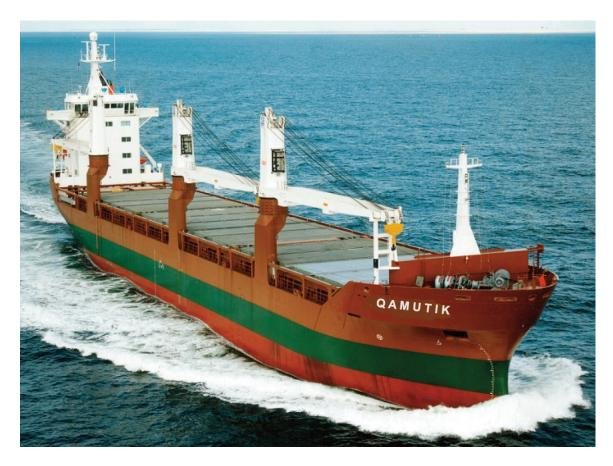
The MV QAMUTIK is the latest addition to NEAS' growing fleet of modern vessels serving Canada's Arctic communities. At 137 meters length, the new vessel is an ice class 1, multi-purpose, tweendecker that offers specialized cargo and advanced handling technologies.
